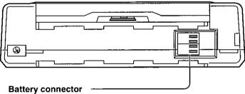
Connect the battery pack [supplied or optional (model No.: DY-DB50EX)]. (See page 25.)
